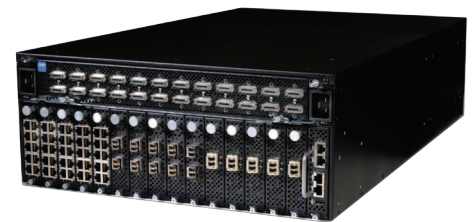
The Xsigo VP780 I/O Director consolidates server I/O by replacing a server’s multiple Ethernet and Fibre Channel interfaces with a single high-speed low-latency link.
